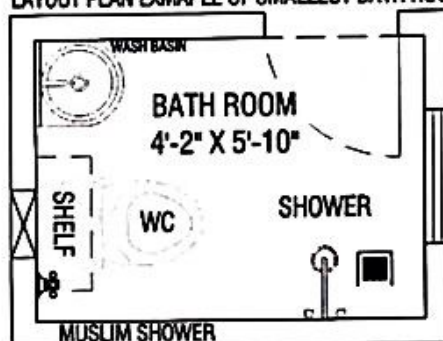
LAYOUT PLAN EXMAPLE OF SMALLEST BATH ROOM
